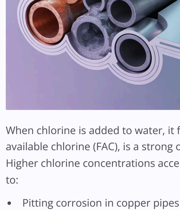
When chlorine is added to water, it forms hypochlorous acid and hypochlorite ion—the active forms known as free available chlorine (FAC), is a strong oxidizing agent that directly attacks metal surfaces in pipes, valves, and fittings. Higher chlorine concentrations accelerate the oxidation of iron, copper, and lead in distribution systems, leading to:
